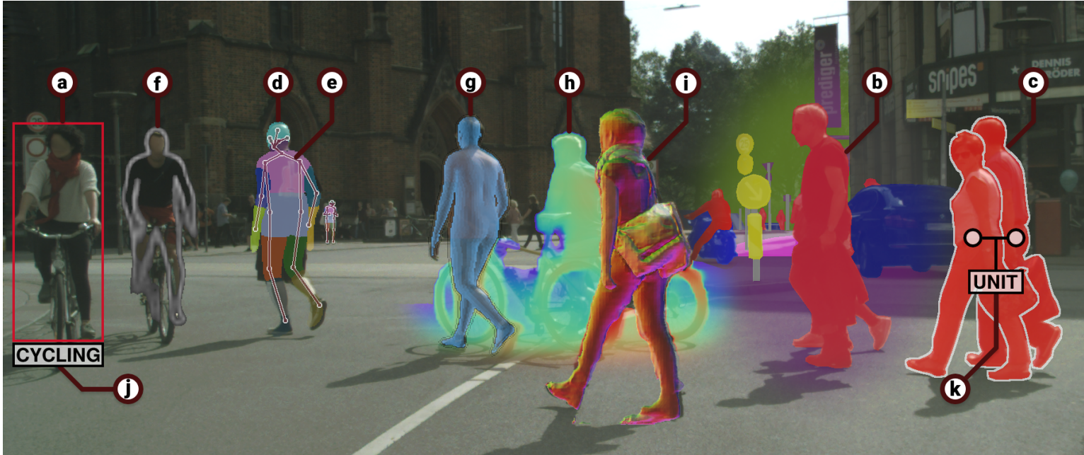
Figure 1.1: What often distinguishes many tasks in human-centric computer vision is the output abstraction extracted from the image. This includes (a) bounding boxes, (b) per-class collections of pixels, (c) per-instance masks — sometimes with (d) fine-grained semantic labels, (e) skeletons both 2D and 3D, (f) 2D contours, (g-i) a variety of 3D surface representations, as well as high-level semantic outputs such as (j) activities or (k) social relations and signals. (See main text for explanations and references.)
