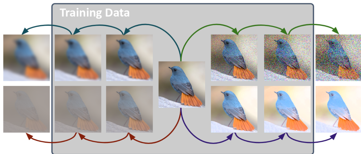
Figure 10.3: Many image transformations that can occur in practice, such as noise, blur, changes in contrast and brightness (depicted above) but also geometric transformations such as scaling and rotation, can be approximated by the repeated application of simple operations. While current recognitions models can learn to handle these given the right data distribution, they struggle when faced with an unseen transformation. Models with inductive biases that allow for learning and recursively applying the inverses of such operations might overcome this limitation.
