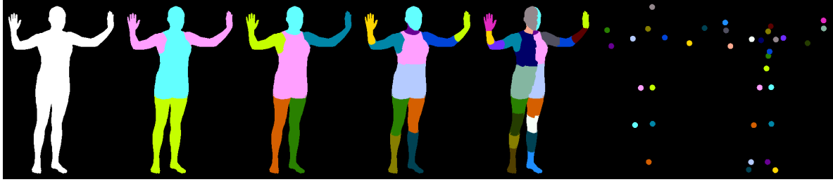
Figure 9.3: Example training image annotations illustrating different types of inputs at different levels of granularities. We generate these automatically from the corresponding 3D ground truth if available. From left to right: 1-, 3-, 6-, 12-, and 24-part segmentations, followed by 14- and 24-joint skeletons.
