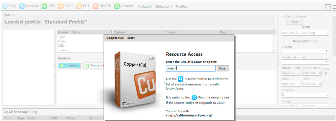
Figure 20. The Copper client environment used for testing CoAP messages.
