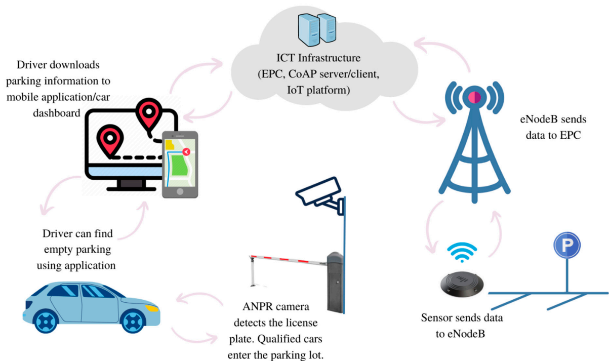
Figure 18. A scenario involving the use of the proposed solution for smart parking.
