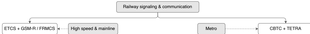
Fig. 2. Main railway signaling and communication systems in railway market segments of interest (in gray)
