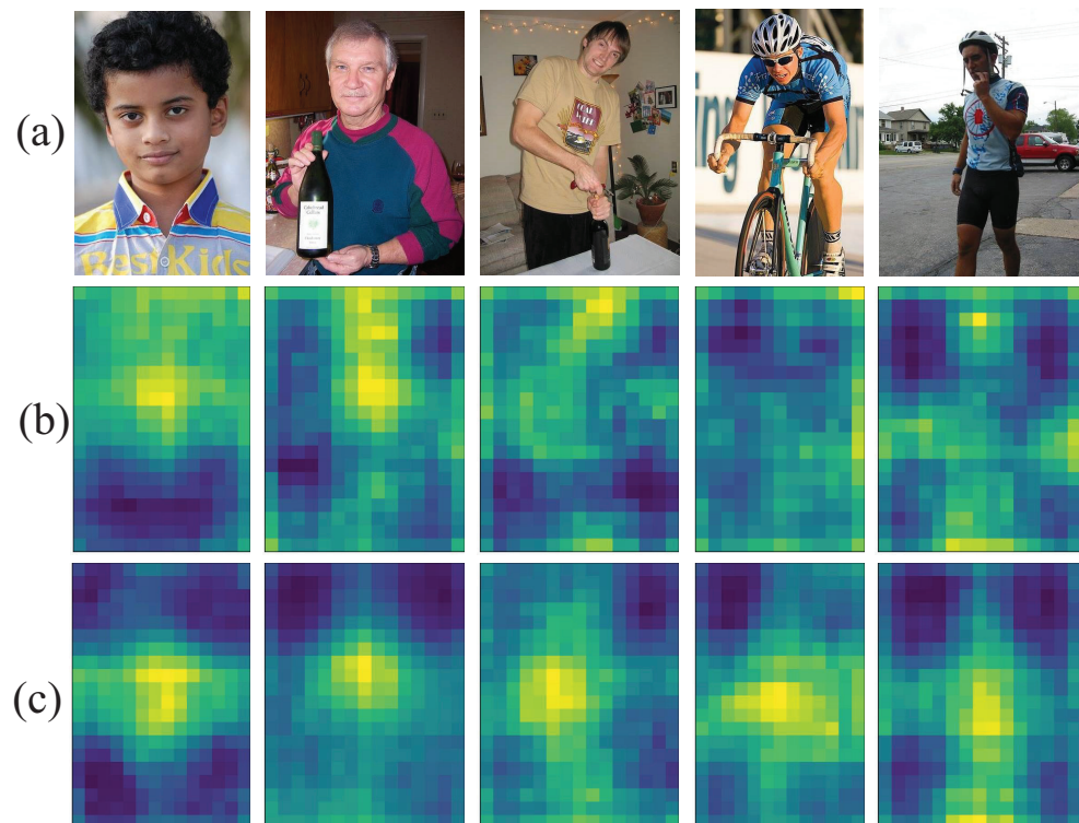
Figure 7. Feature visualization comparison of the last layer of the backbone network between YOLOv5s and CA-YOLOv5s. (a) Input image. (b) Feature visualization of C3 in YOLOv5s. (c) Feature visualization of CA in CA-YOLOv5s.
