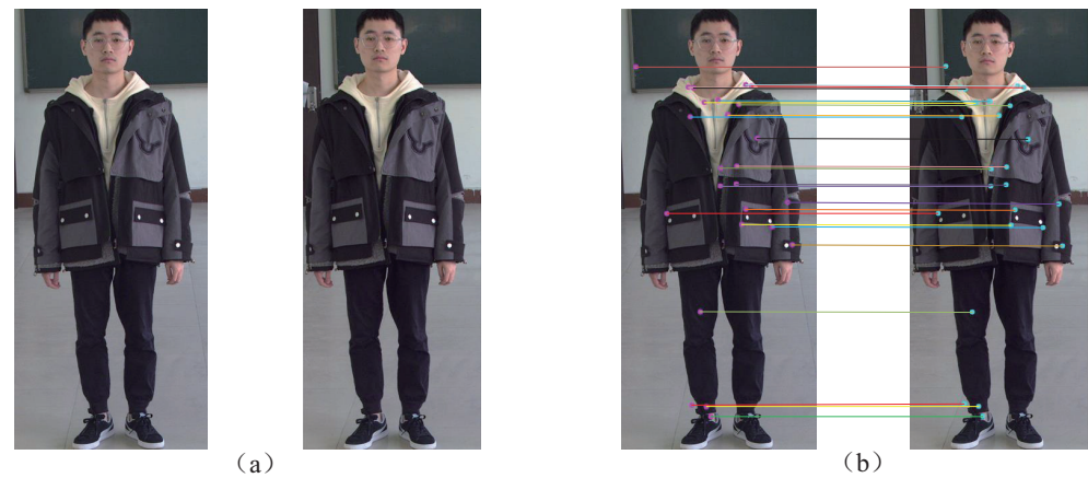
Figure 9. A pair of extracted pedestrian regions and their matching results. (a) Pedestrian region pair. (b) Matching results.
