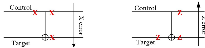
Figure 2. Schematic diagram of the error propagate of CNOT gate, where an X error propagates from the control qubit to the target qubit and a Z error propagates from the target qubit to the control qubit.
