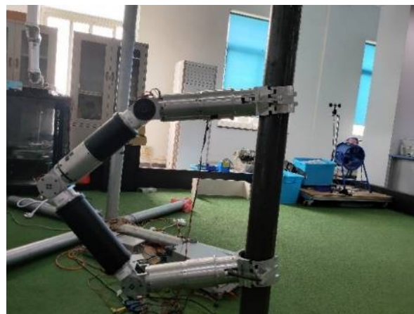
Figure 7. Schematic diagram of the inchworm robot climbing scene.
