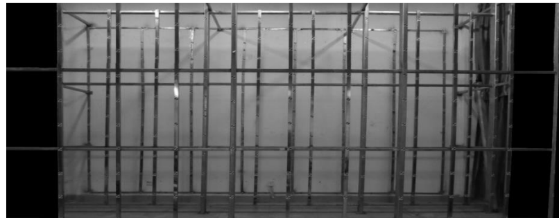
Figure 8. The DOM generated by the method above for the indoor 3D calibration field.
