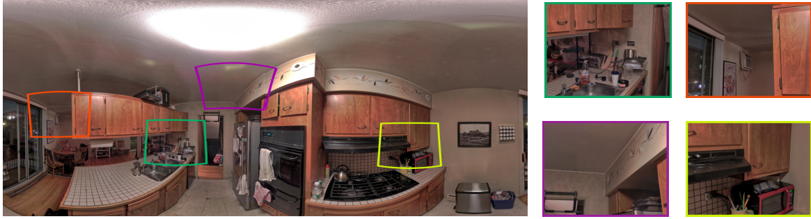
Figure 2.4: Illustrations of image/depth map cropping and rectification process. Left: a panorama (approx. 8K \times 20K pixels) produced by the scanner; every pixel with a valid return is associated with a depth value. Four colored frames indicate a subset of FOV crops projected on the panorama. Right: the corresponding frames after reprojection (to correct artifacts like those on the soffit in the purple frame), downsampling to 768 \times 1024 pixels, and rectification. The depth map associated with the panorama is cropped and rectified in the same way, yielding aligned RGB-D pairs.
