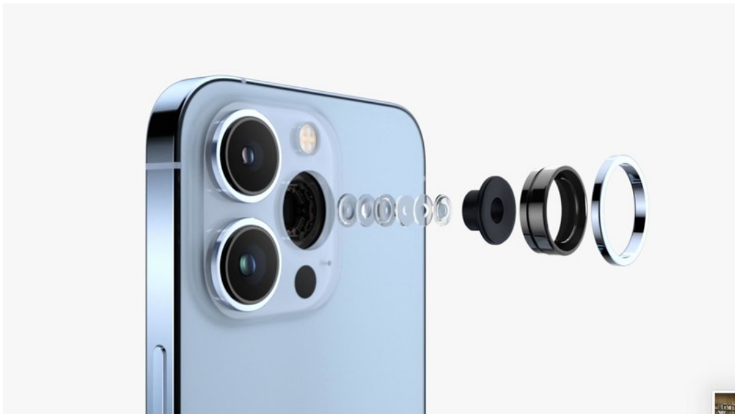
Figure 2.1: Modern smartphone cameras use a complex series of lenses to focus light on their tiny sensors.
