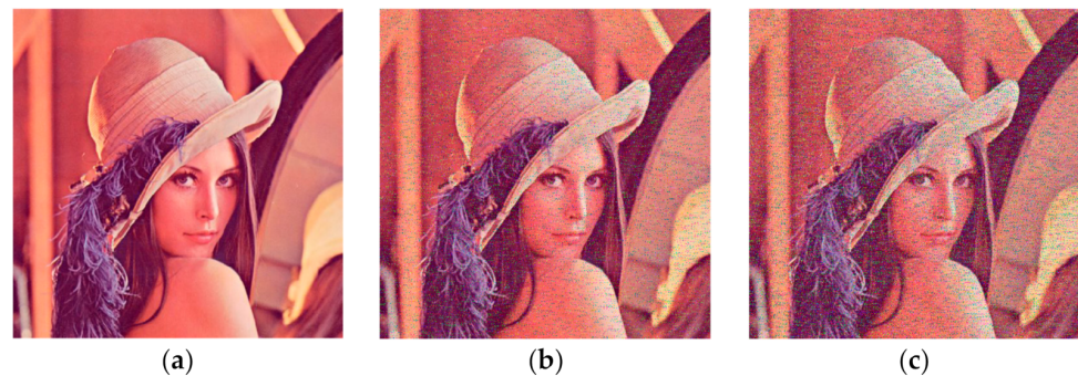
Figure 13. Decryption results for encrypted image: (a) without adding noise; (b) with 0.05 density noise; (c) with 0.2 density noise.
