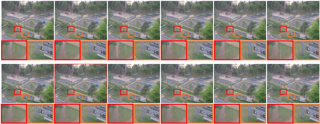
Figure 8.9: Deraining results on the real-world rainy sequences. The top and bottom rows are the input sequences and the output sequences from our proposed model, respectively. Best viewed in color.
