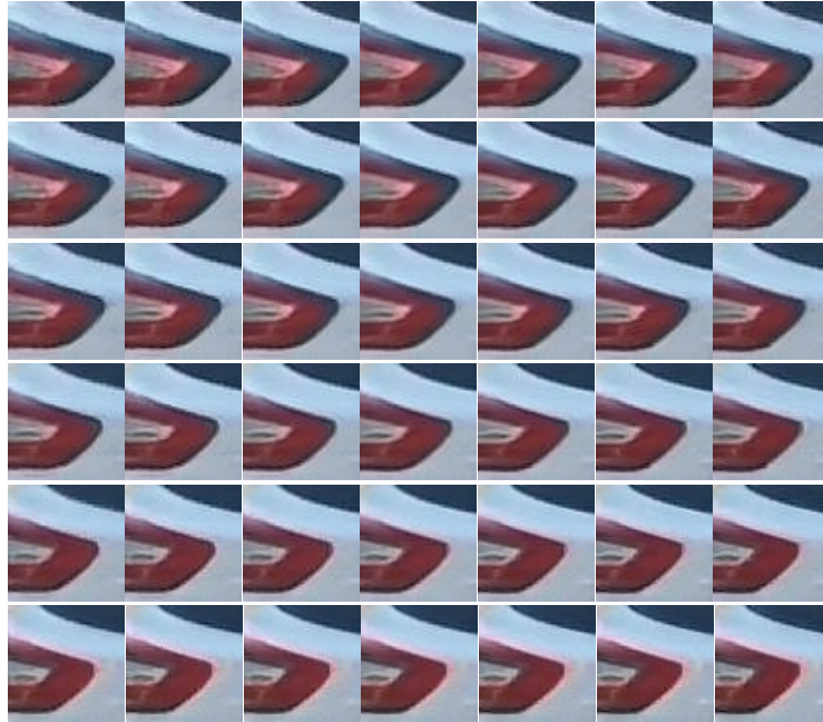
Figure 5.7: Example of interpolation of subtle motions. 42 frames (from left to right, top to bottom) are extracted by the proposed method based on the input image shown in Fig. 5.1. Please check the movement of the rear light comparing the first frame with last one. Note that there are no 42 original frames as the input blurry frame is produced by averaging only 7 frames. By iteratively applying the model we are therefore able to create slow-motion videos from blurry images.
