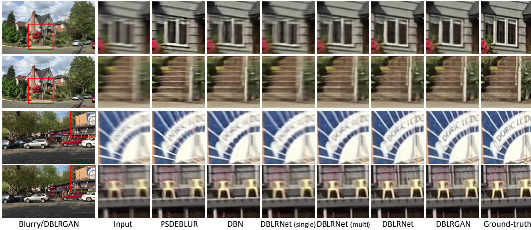
Figure 4.4: Exemplar results on the VideoDeblurring dataset (quantitative subset). From left to right: real blurry frame/ Output of DBLRGAN, input, PSDEBLUR, DBN [Su et al., 2017a], DBLRNet (single), DBLRNet (multi), DBLRNet, DBLRGAN and ground-truth. All results are obtained without alignment. Best viewed in color.
