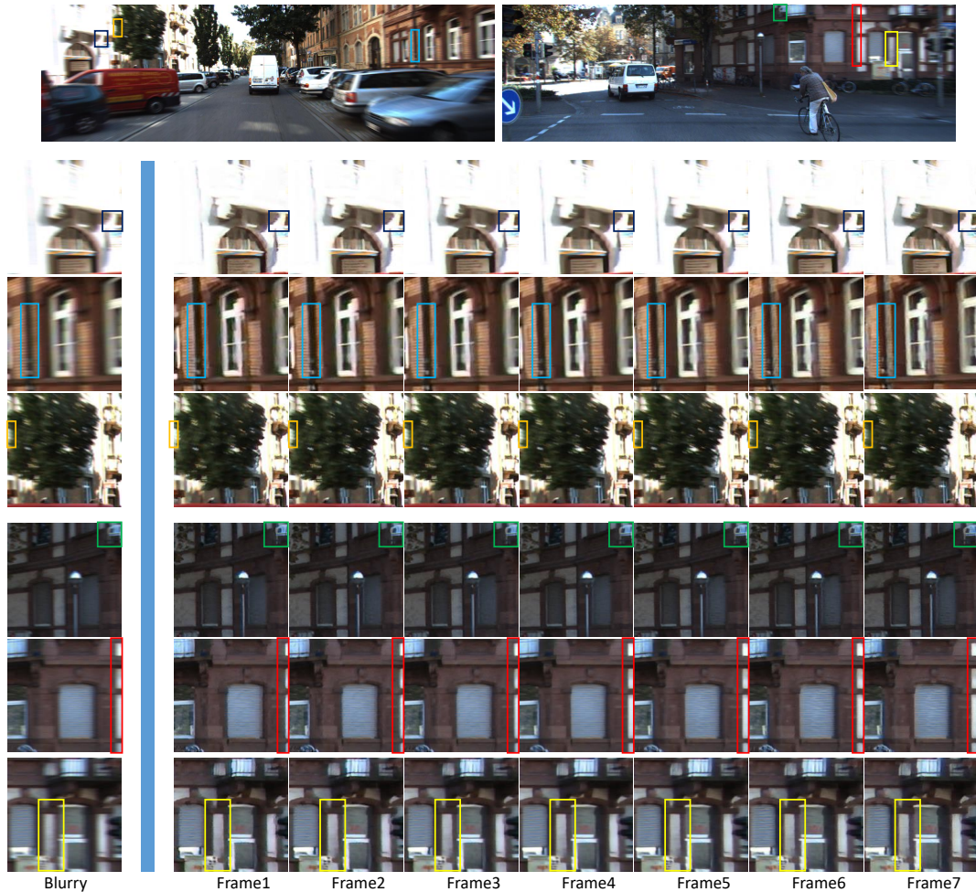
Figure 5.9: Results on the KITTI dataset. The first column shows details of the two blurry input images in the top row, and the following seven columns show images generated by the proposed model. The subtle motion outlined by boxes with different colors shows that the model generalizes well to blur caused by bokeh.
