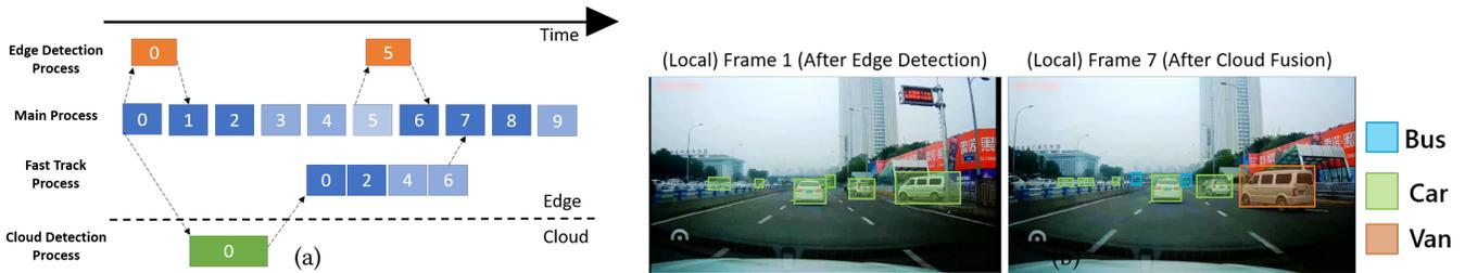
Figure 2: (a) REACT System Process Flow. Orange and Green boxes indicate edge and cloud detections, respectively. Tracking performance degrades with streaming age, which is indicated by the lighter shades of the color blue. It should be noted that Cloud Detection and Fast Track are both asynchronous events. (b) REACT uses asynchronous cloud detections to correct the box labels and detect more objects.
