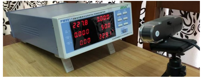
Fig. 15. Energy data are collected using a power meter and a webcam.
