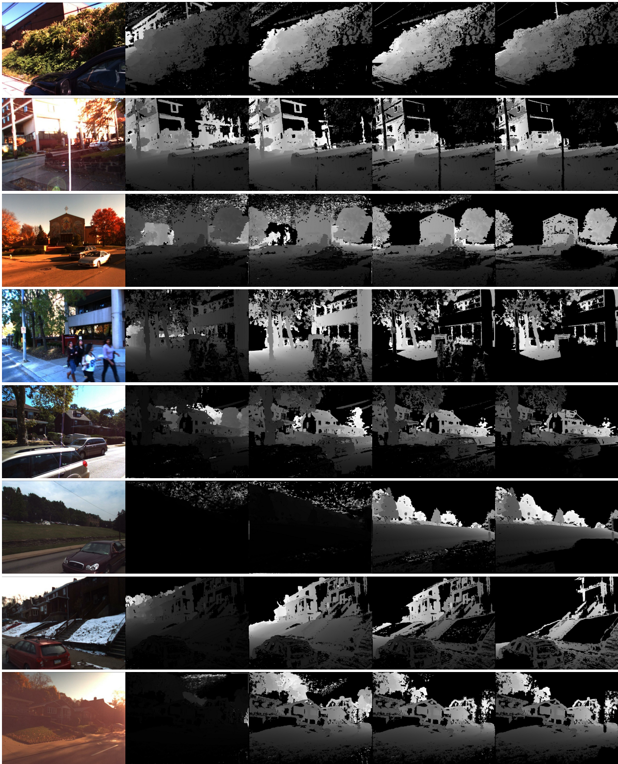
Figure 9. The processing samples given RGB image followed by normalized depth maps for clear visualization of (a) dense reconstruction, (b) range filtering, (c) HSV-based refinement and (d) manual post-processing.
