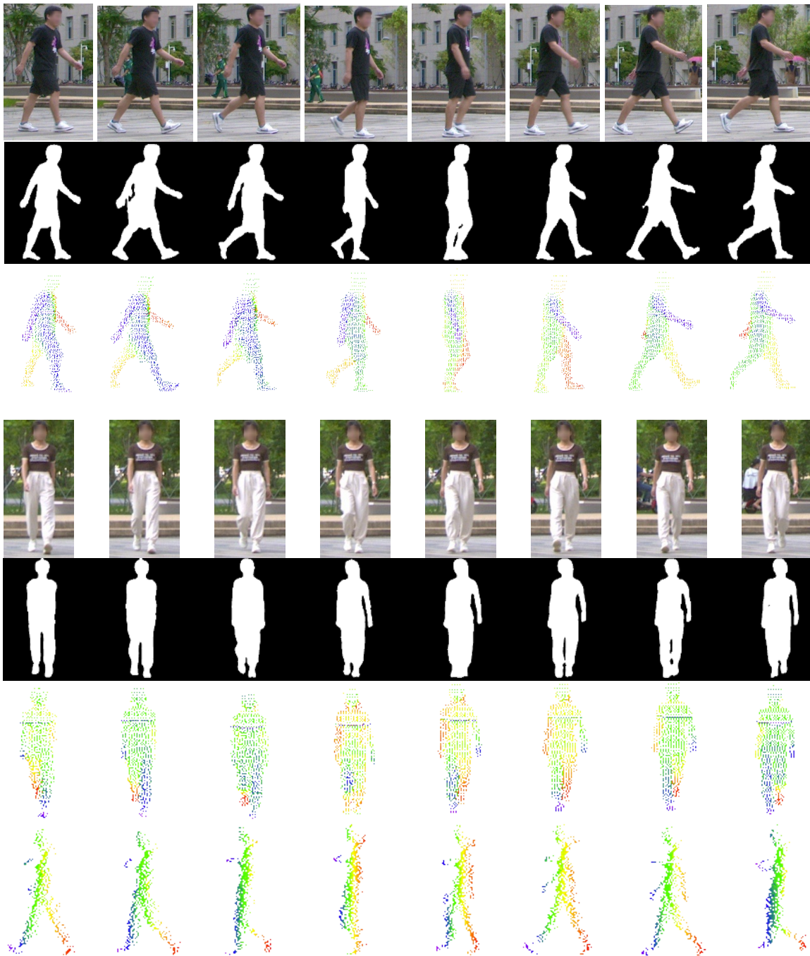
Figure 13. Exemplar sequences of LIDAR GAIT dataset under normal conditions. Eight frames in three modalities are visualized. The top three rows show three gait representations in RGB images, silhouettes, and point clouds. The bottom four rows represent gait representations in RGB images, silhouettes, front-view point clouds, and side-view point clouds. It shows Lidar provides informative 3D geometry. (Best viewed in color.)
