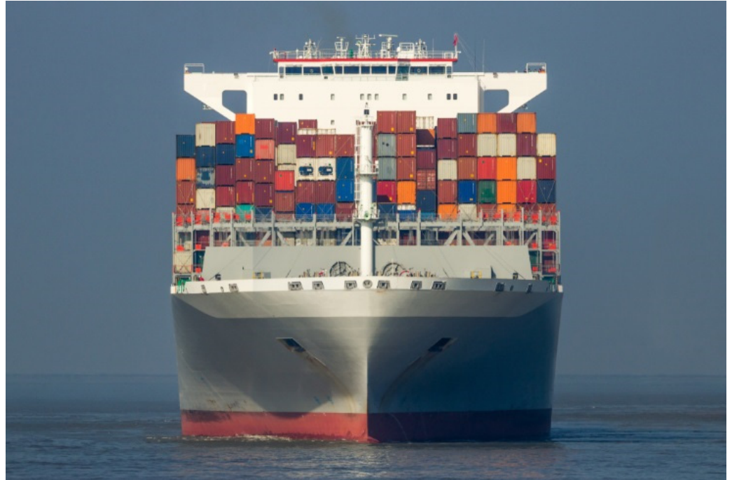
Figure 37. The profile of a large container ship from a forward view. While the angled hull presents a lower drag coefficient, most of the above-deck structure and load offer high resistance.
