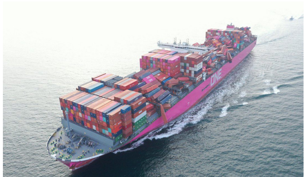
Figure 31. The ONE Apus arrives in Kobe, Japan, on 8 December 2020 after losing an estimated 1816 containers overboard, approximately 1600 nautical miles northwest of Hawaii, USA. Photo courtesy W K Webster and Co. Sidcup, UK.
