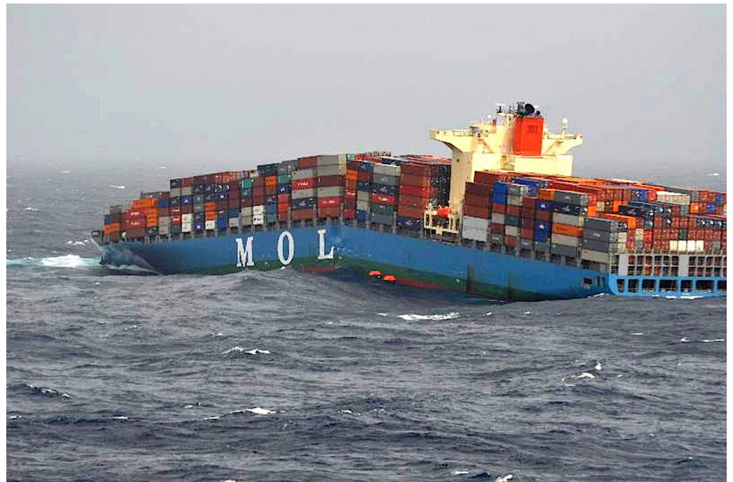
Figure 30. Breakup of the container ship MOL Comfort, off Yemen, in June 2013. Photo from [109] with permission; originally taken by Mitsui O.S.K. Lines, Ltd., Tokyo, Japan.
