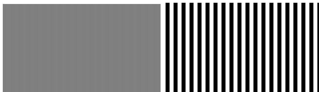
Figure 2. Stripe patterns in different colors. The difference between two adjacent stripes on the left is 1, while the difference on the right is 255.
