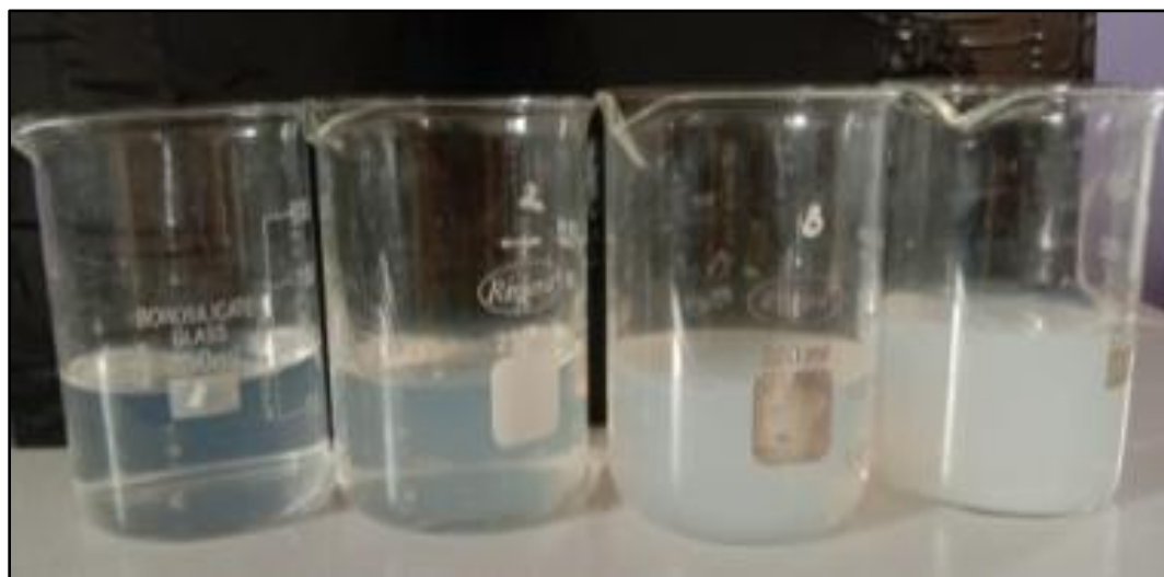
Figure 1. Photograph of silica gel prepared using different concentration of sodium silicate
