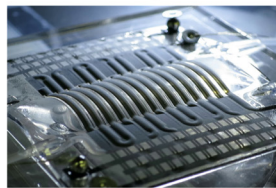
Slug drive micro-conveyor with 28 actuators
