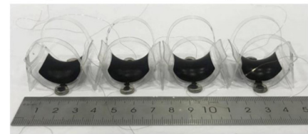
1-by-4 annelid-like crawling robot
