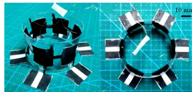
1-by-6 multi-segment annular robot
