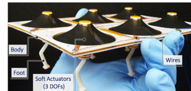
Multiple-degrees-of-freedom hexapod robot
