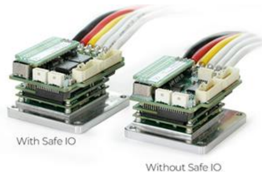
Figure 5 "Platinum Solo Twitter" DC servo drive (ELMO Motion Control)
