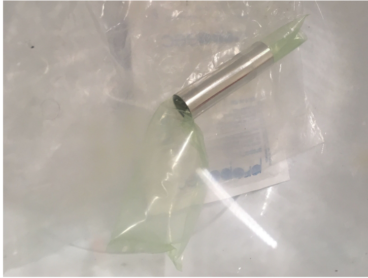
Figure 53: Testing of inflated pressure bag (green-ish) inside an aluminum tube
