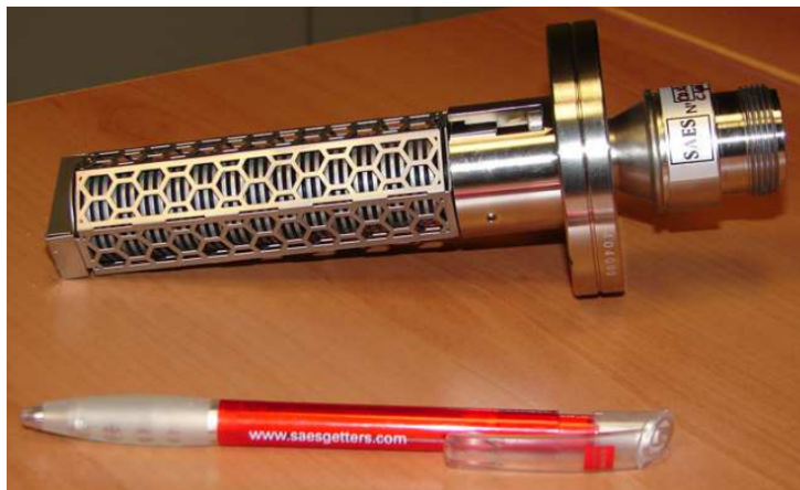
Figure 27: Dimensions of a NEG Pump [ HandbookVacuumtech16 ]
