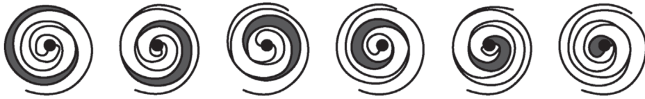
Figure 25: Functioning principle of a scroll pump [HandbookVacuumtech16]
