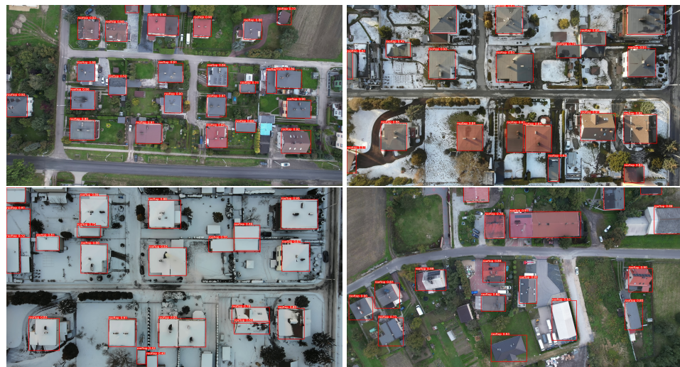
Figure 7. Results of the roof detection algorithm under different weather conditions.
