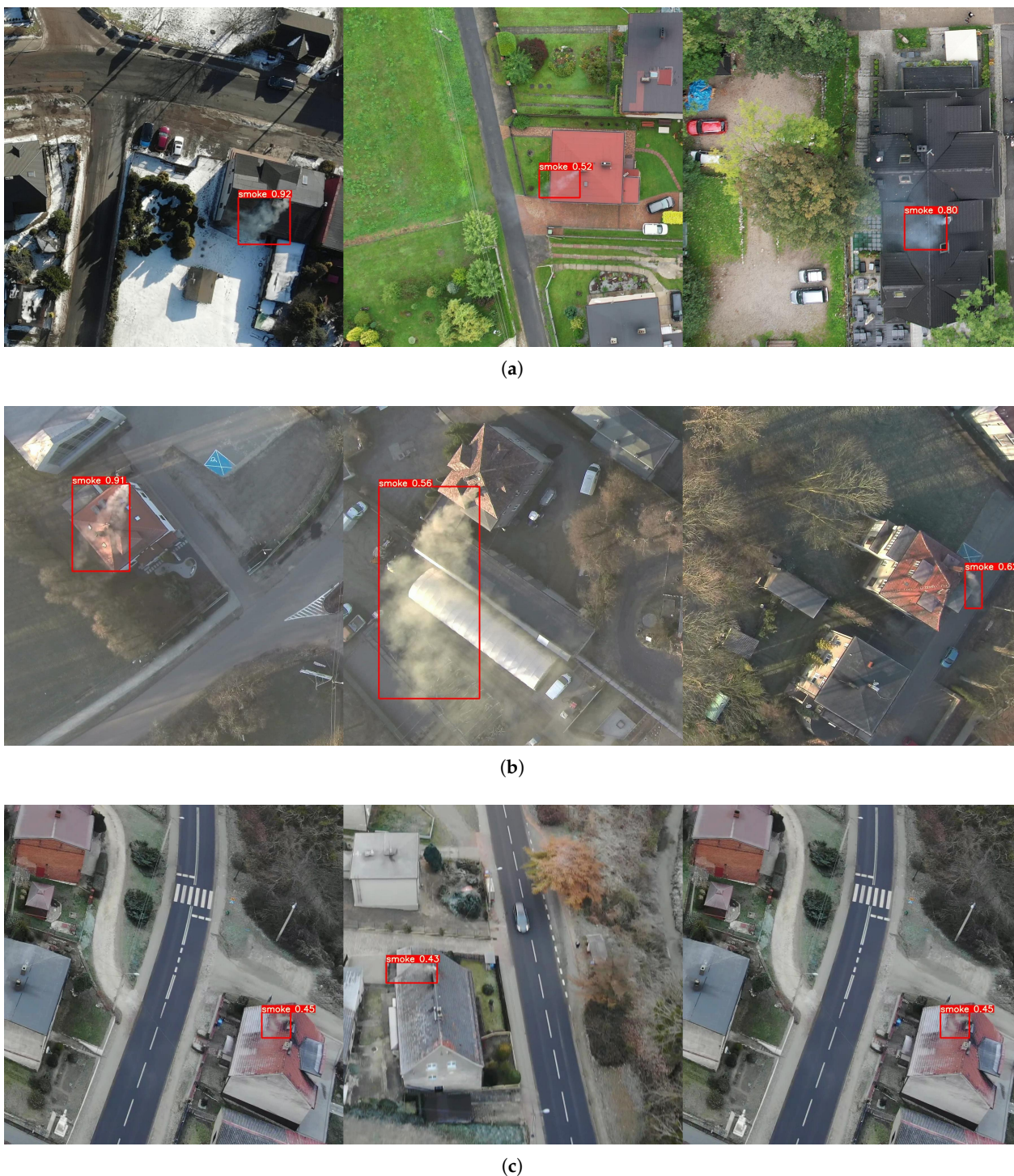
Figure 10. Example detection results for the YOLOv7-x model. (a) Detections from DJI Drones; (b) Detections from Xiaomi Mi Drone Video; (c) Detections for oblique flight.
