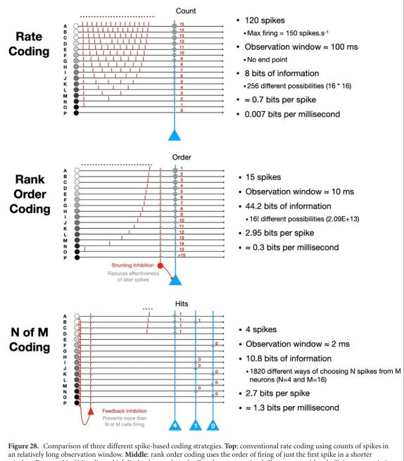
window. **Bottom**: N of M coding which limits the number of spikes that a transmitted allows very rapid and efficient transmission of large amounts of data.
