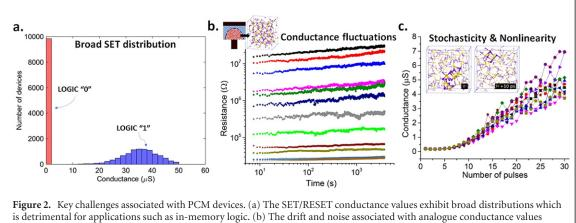
is detrimental for applications such as in-memory logic. (b) The drift and noise associated with analogue conductance values results in imprecise matrixvector multiply operations. (c) The nonlinear and stochastic accumulative behaviour result in imprecise synaptic weight updates.
