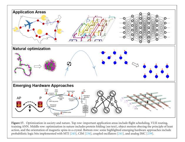
ferromagnetic and antiferromagnetic coupling using simple electrical elements such as resistance and capacitance, and can achieve highly parallelized all-to-all connectivity. The analog or continuous-time dynamics of these Ising solvers has an inherent advantage of parallelism which lowers the time to solution compared to CMOS annealers and CPUs operating in discrete time. The time-to-solution (or cycles-to-solutions) remains similar for both the IMT solver and RRAM-based hardware accelerator.
