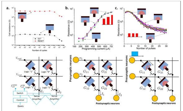
**Figure 1.** Key physical attributes that enable neuromorphic computing. (a) Non-volatile binary storage facilitates in-memory logical operations relevant for applications such as hyper-dimensional computing. (b) Analog storage enables efficient matrix-vector multiply (MVM) operations that are key to applications such as deep neural network (DNN) inference. (c) The accumulative behaviour facilitates applications such as DNN training and emulation of neuronal and synaptic dynamics in SNN.
