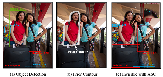
Fig. 1: We conduct a sparse attack on object detectors guided by a contour prior, which can be rough and outlined manually. With pixel sampling and texture optimization, we successfully make the woman in the green bounding box invisible to DETR (Carion et al., 2020), while other objects remain detectable, by modifying only 2% of the pixels in the object area.
