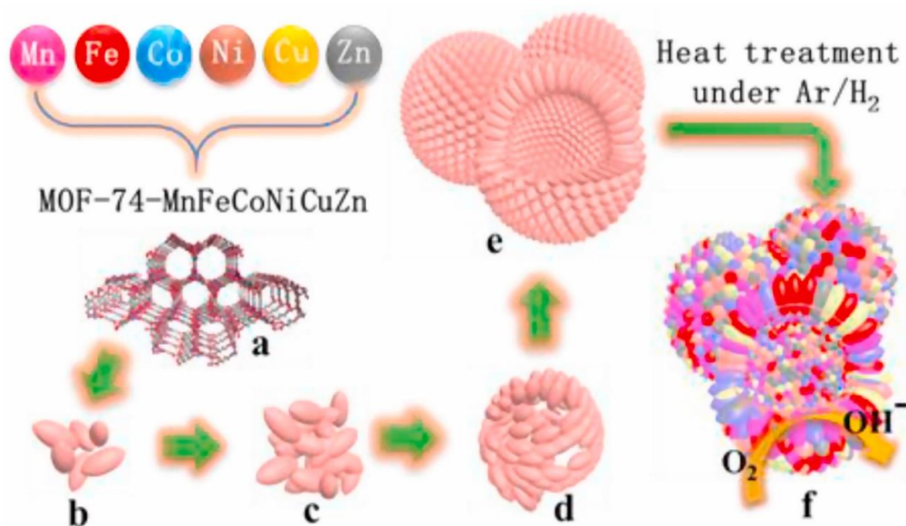
Figure 21. Schematic diagram of porous hollow high-entropy alloy catalyst production. (a) Crystal structure of MOF-74-H. (b) Small number of MOF particle aggregated. (c) Large number of MOF particle aggregated. (d) Secondary nucleation. (e) Dissolution regrowth-formation of hollow multi-metal-organic framework. (f) Hollow metal/metal-alloy/metal-oxide (MOF-74-H-650) nanocomposite for ORR. (Reprinted with permission from [281]. Copyright 2021, Elsevier).
