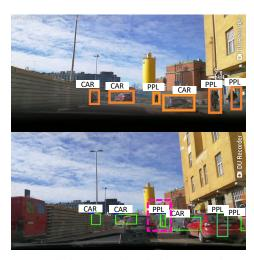
Figure 14: A depiction of a simplistic cooperative perception system. A vehicle in the lead identifies things indicated by orange bounding boxes (top figure). These objects are displayed in green bounding boxes to the driver of the following vehicle (bottom figure). AICP filters these items to only display critical ones (such as the pedestrians in the pink bounding box) in order to limit the number of objects displayed on-screen.
