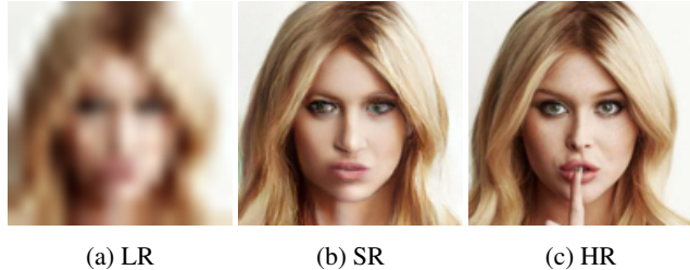
Figure 3: A Comparison of a LR, SR, and HR image (CelebA-HQ) illustrates the quality of our proposed method for the 16 \times 16 \rightarrow 128 \times 128 setting. The LR image shows a significant loss of information, particularly the presence of a finger in front of the mouth. Our proposed method can reconstruct the image with great detail, particularly in the hair. However, the HR image shows that our method cannot reconstruct the finger. Also, the HR image shows more defined edges and sharper details of the eyes.
