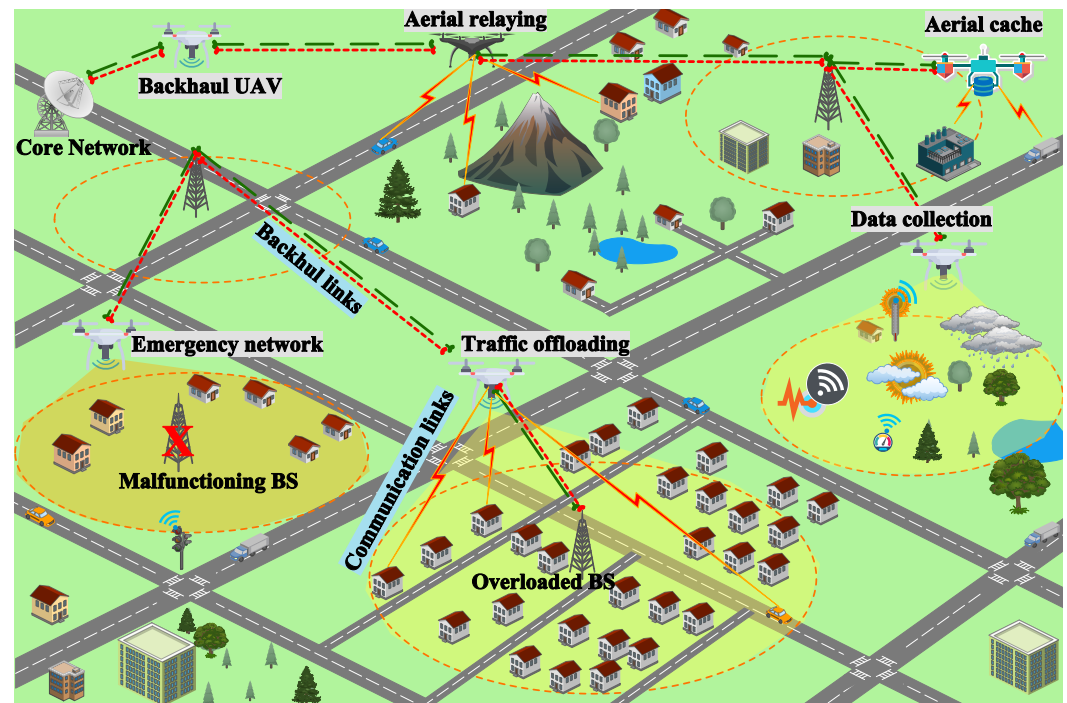
Figure 4. Different UAV use cases involving the UAV serving as a wireless backhaul to connect users located in remote areas to the core network, as a emergency network for restoring service to an area covered by a malfunctioning BS, as a aerial relay for providing coverage extension to users separated by obstacles such as hills and mountains, data offloader for offloading user traffic from overloaded terrestrial BSs to ensure load balancing and throughput enhancement, as aerial cache for serving popular content to ground users to reduce backhaul congestion and achieve EE and as a data harvester for collecting data from ground sensor nodes.
