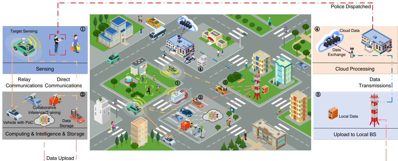
Fig. 1. VaaS for public safety. In the figure, a crime scene is video-recorded from different angles and collaboratively analyzed by surrounding vehicles (both moving and parked vehicles), based on multi-modal sensing and collaborative perception. The summarized results will be transmitted to the police department for further action.
