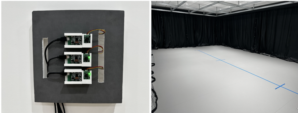
Figure A.1: This figure presents a dual-view illustration. The left panel shows a wall-mounted sensor assembly, consisting of sensors developed by Harvard on the left side and those provided by Useful Sensors on the right. The right panel depicts the experimental environment where study participants stood in front of the sensor setup. Distances from the sensor setup (1m, 3m, and 5m) are marked on the floor for participant positioning.
