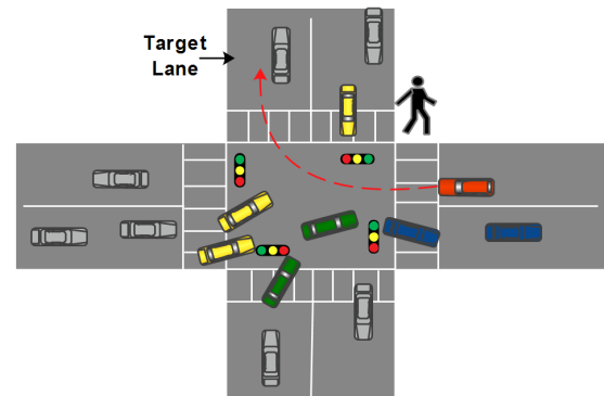
Fig. 20: Depiction of the intersection scenarios: The Ego-Vehicle, represented by the Red vehicle, is about to change lanes to the target lane. To ensure socially acceptable driving behavior, the Ego-Vehicle must anticipate the future movements of the yellow vehicles. This prediction also includes taking into account the presence of green vehicles.
