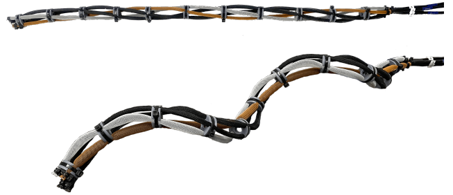
Fig. 1: The HISSbot uninflated (top), and pressurized to form a helical shape for sidewinding (bottom). Cyclical contraction of the four McKibben actuators produces locomotion via a twisting-helix motion.
