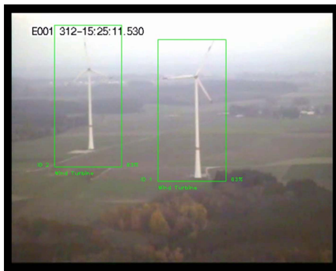
Fig. 10. Wind turbine detection from the FTI camera.
