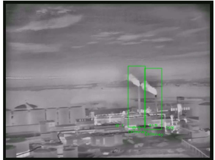
Fig. 13. Chimney detection from the HeliEVS camera.
