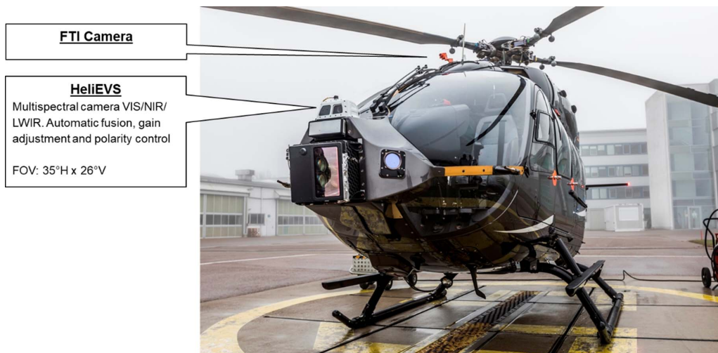
Fig. 7. FTI and HeliEVS sensor installations on an experimental H145 helicopter.
