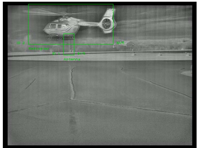
Fig. 14. Antenna and helicopter detection from the HeliEVS camera.
