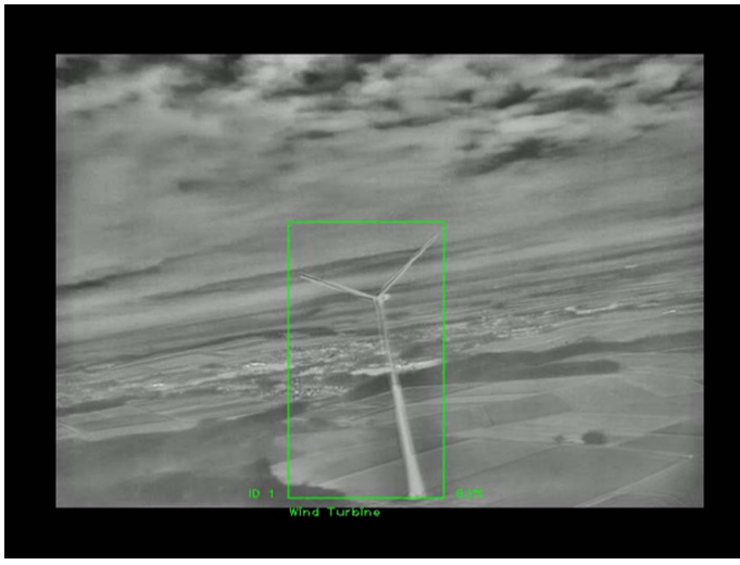
Fig. 11. Wind turbine detection from the HeliEVS camera.
