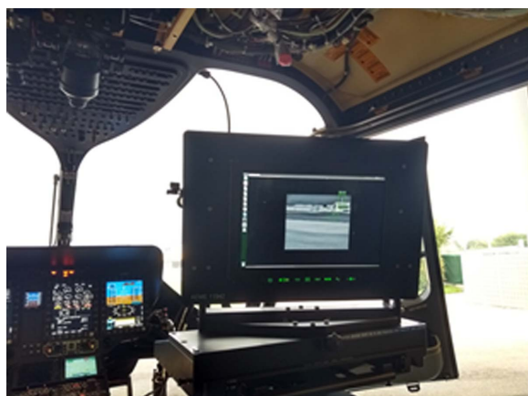
Fig. 9. Real-time display of the CNN+SVM output in the operator cabin console.
