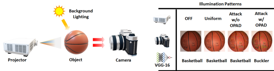
Fig. 7. The framework of adversarial light projection. Due to the background lighting, the table shows only projecting the adversarial illumination with environment loss compensation can successfully fool the VGG-16. This figure is from [48].
