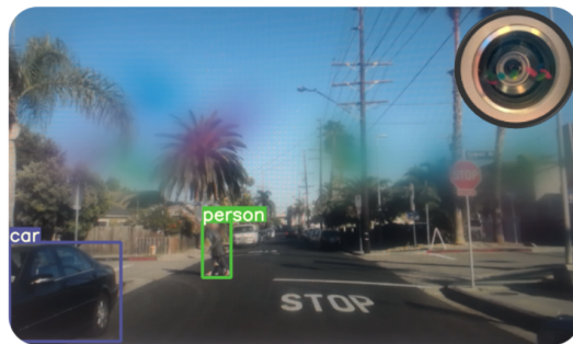
Fig. 8. Translucent patches are stuck to the camera lens and successfully hide the stop sign under the detector. This figure comes from [173].
