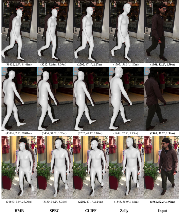
Figure 7: Qualitative results for 3DPW. Zolly achieves good alignment with the characters in the original image, but other SOTA methods have difficulty aligning images that suffer from distortion caused by overhead shots, which causes upper body dilation and lower body shrinkage. The number under each image represents predicted/ground-truth f , FoV angle, and T_z .
