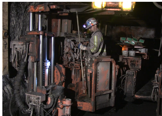
Fig. 5: A human operator is installing a bolt into the roof bolter. 2
