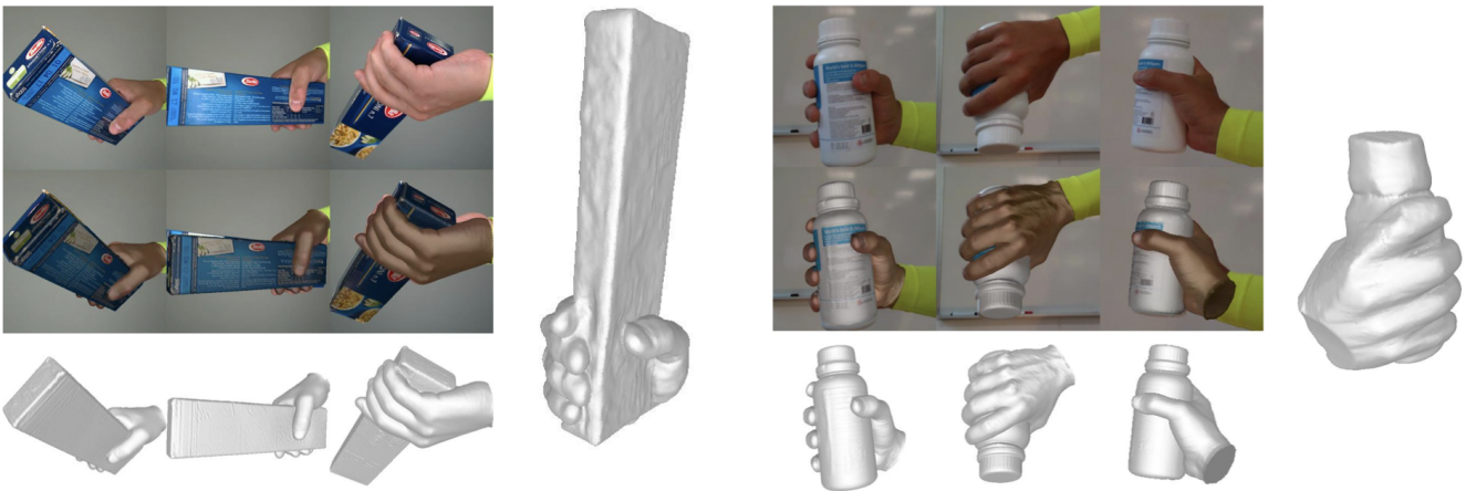
Figure 1: The SHOWMe dataset comprises 96 videos with their associated high-quality textured meshes of a hand holding an object. For two different samples, we show on the left side, row by row, real RGB crops from the dataset, an overlay of the corresponding ground truth textured mesh, and a rendering of the texture-less mesh with Phong shading. On the right, we show the 3D reconstruction of the hand-object obtained from the RGB stream only, using one of the evaluated baselines.
