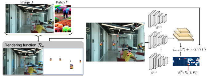
Fig. 6: The pipeline of Facebook's work [119] in training an adversarial patch to attack both YOLO and Faster R-CNN detectors.
