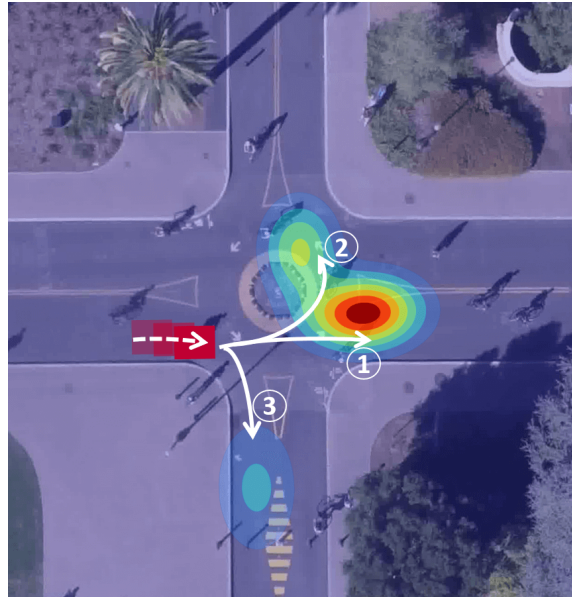
Figure 4.47: Presence of aleatoric uncertainty in future prediction. “Given the past images, the past positions of an object (red boxes), and the experience from the training data, the approach predicts a multimodal distribution over future states of that object (visualized by the overlaid heatmap). The vehicle is most likely to move straight (1), but could also continue on the roundabout (2) or turn right (3).” [135] Figure taken from [135].
