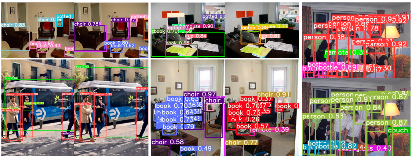
Figure 9. The comparison of the detection results of the two algorithms on the test samples. The left and right side show the comparison of target detection results between YOLOv5s and GS-YOLOv5s. In the last figure, the top is YOLOv5s's results, and the bottom is GS-YOLOv5s's.
