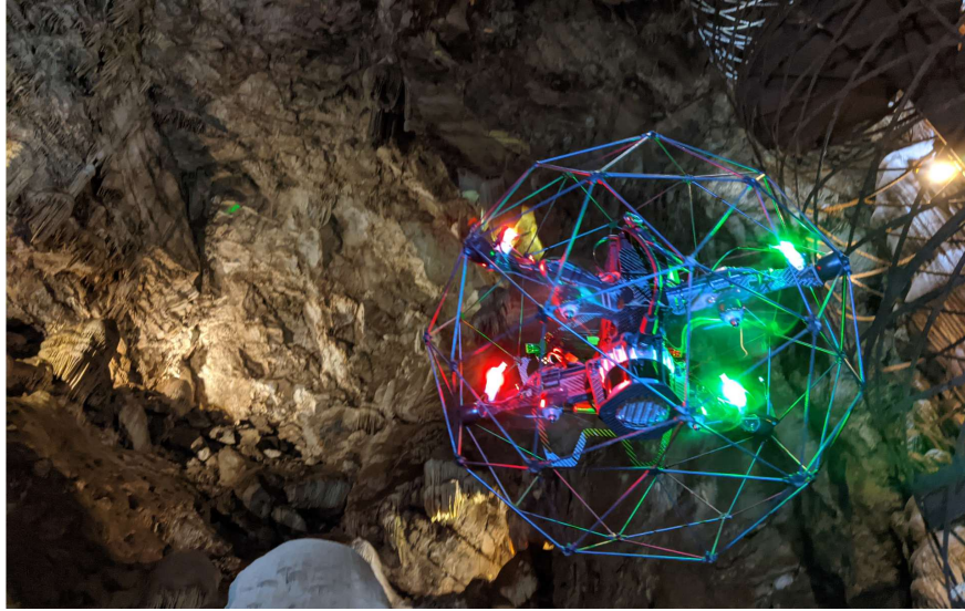
Fig. 3 Example of a collision-tolerant aerial robot: The Gagarin system (Dharmadhikari et al 2020a) tested in subterranean environments.
