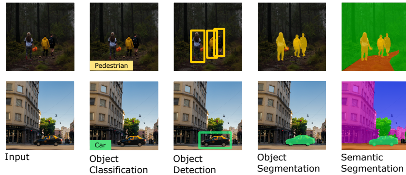
FIGURE 1.1 Each row shows an example with an input image and the corresponding output of different scene understanding tasks. Object classification identifies "what" objects compose the image, object detection predicts "where" the objects are located in the image, object segmentation outputs a mask that indicates the shape of the object. Semantic Segmentation further details the input image by predicting the label of all the pixels, including the background.
