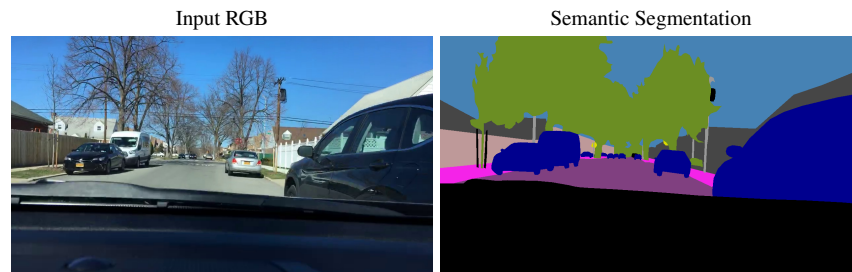
FIGURE 1.11 An example of semantic image segmentation from the challenging BDD100K dataset. The image shows a complex urban scene with many dynamic objects.
