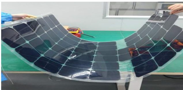
Fig. 5. Flexible solar panels of our airship.
