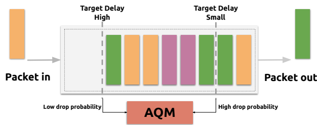
Figure 1: The trade-off: If the Target Delay is small, can increase packet losses and decrease link utilization. If is high, increase queuing delays and decrease packet drops.
