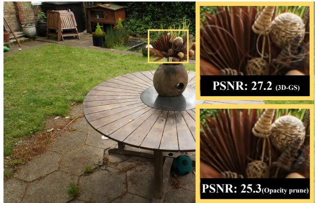
Figure 3. Zero-shot Opacity-based Pruning. A significant number of Gaussians exhibit small opacity values (top). Simply utilizing Gaussian opacity as an indicator for pruning the least important Gaussians results in the rendered image losing intricate details (bottom), with the PSNR dropping from 27.2 to 25.3. This has inspired us to find better criteria to measure global significance in terms of rendering quality. The accumulated PDF is equal to 1.
