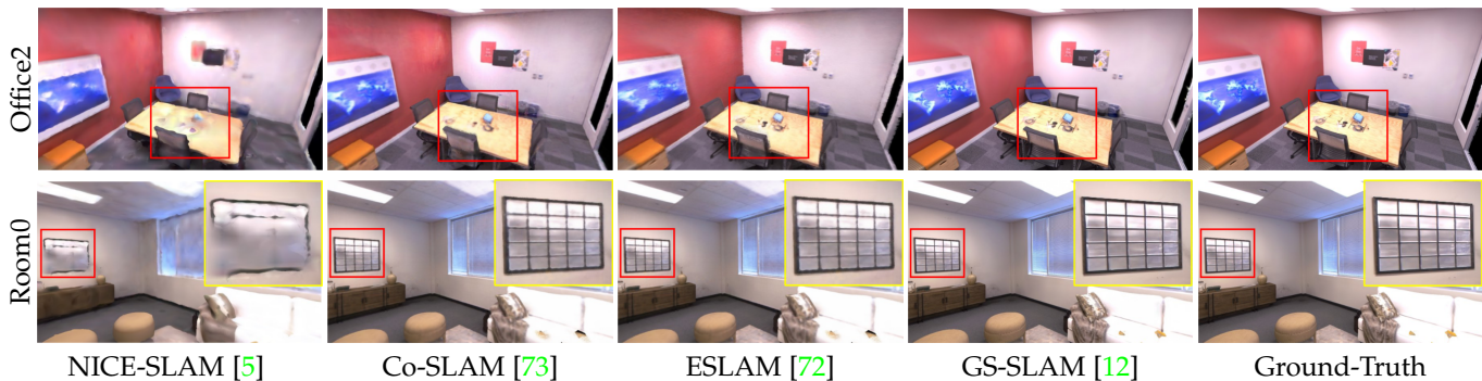
Fig. 14: SLAM Methods Comparison on the Replica [68] Dataset– Image Rendering. Images sourced from [12].
