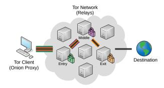
Figure 1: Tor network. Traffic is relayed via three Tor nodes to hinder correlation of the client and the destination.
