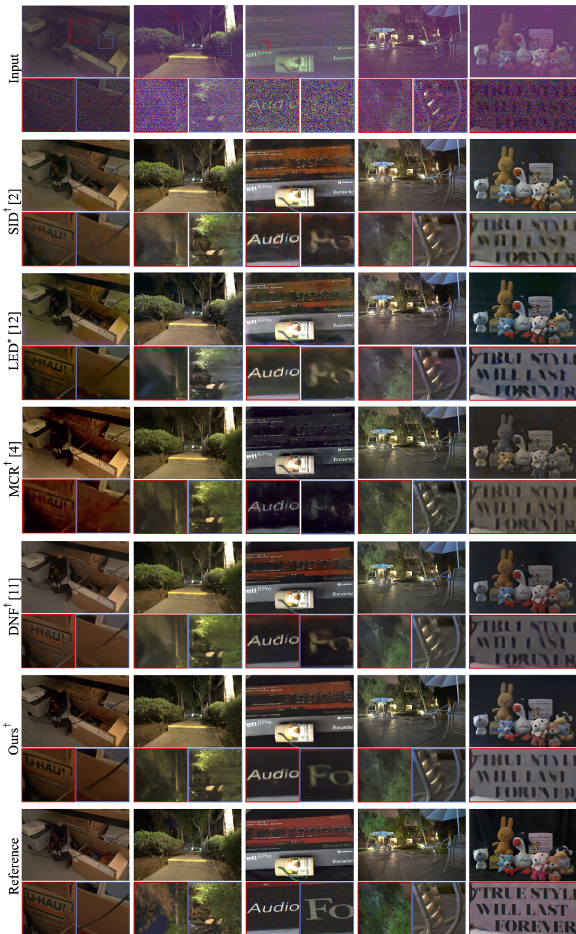
Fig. 5: The qualitative evaluations on SID-Sony [2] and ELD-Sony [30] datasets (Zoom-in for best view). The proposed method shows notable superiority in recovering structural information and enhancing details in extremely dark and noisy regions. († denotes the RAW-to-sRGB method and * denotes the RAW-to-RAW method)
