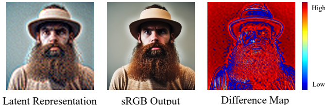
Fig. 3: A text-to-image example from a well-known latent diffusion model, Stable Diffusion. The difference map between the latent representation and sRGB output indicates that the latent representation generated by the UNet shows essential structural content while the decoder \mathcal{D} introduces abundant details but scarcely modifies the global structure for the final sRGB output. The latent representation is converted to sRGB visualization by the linear transformation [13].
