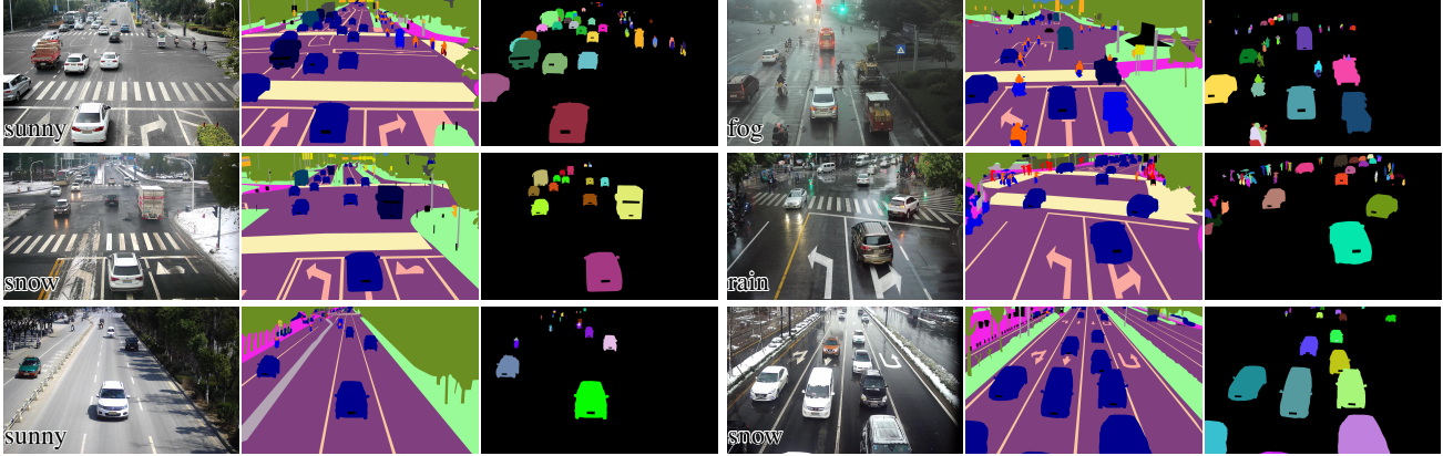
Figure 1. Examples are randomly picked from the TSP6K dataset. Each image is associated with its corresponding semantic label and instance label. We have masked the vehicle plates for privacy protection.
