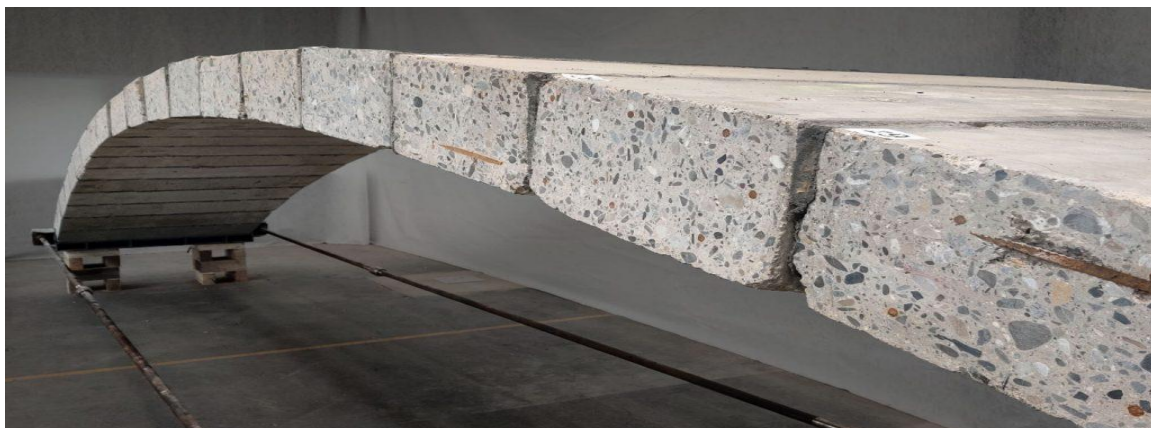
Figure 3 Re:Crete footbridge prototype (source: Devenes et al., 2022)
