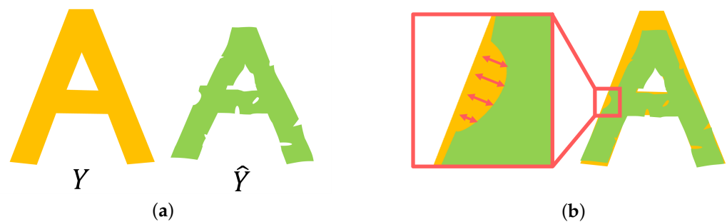
Figure 3. Boundary-based distance between GT and prediction. (a) A GT Y and a prediction \hat{Y} . (b) Overlay of Y and \hat{Y} . Although the GT and prediction are actually binary images, for easy understanding, Y and \hat{Y} are represented in orange and green, respectively. Boundary-based distance focuses on how far apart the pixels of two boundaries are.
